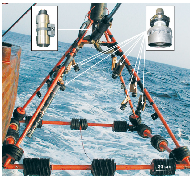
Fig. 3. School for Marine Science and Technology (SMAST) video sampling pyramid aboard the FV 'Huntress'. Pyramid has square base, 2.2 m per side, of 6 cm round iron, arms of 2.5 m × 4.5 cm round iron, and weighs approximately 450 kg. It is deployed with the large hydraulic winch used in the scallop fishing industry while a second tension sensitive hydraulic winch controls the electronic cable. Rubber rings (3 sets of 8 rings, each 20 cm diameter, 5 cm thickness, per side) are placed on the base of pyramid to prevent damage during deployment and provide gentle landing on the sea floor. Underwater camera (insert top left, Deepsea Power & Light® multi-Seacam) and up to nine 100 W lights (insert top right, Deepsea Power & Light® multi-Sealite) were attached to pyramid
