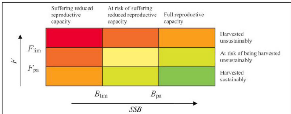
Figure 5.1.1. An overview of the status of fish stocks in relation to reference points, the basic idea being that, to have a high probability of avoiding a stock ending up in the red area (below  $B_{lim}$  and above  $F_{lim}$ ), decisions on management targets should be constrained within the green area (above  $B_{pa}$  and below  $F_{pa}$ ; from Hauge *et al.*, 2007).
