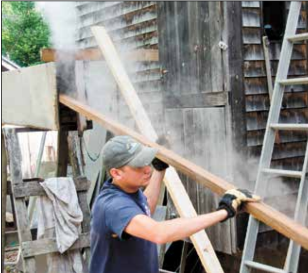
White oak ribs, 1-1/2" x 2-1/2", are heated for two hours in a steam box until pliable. Hustling them to the installation point before they cool is important.
