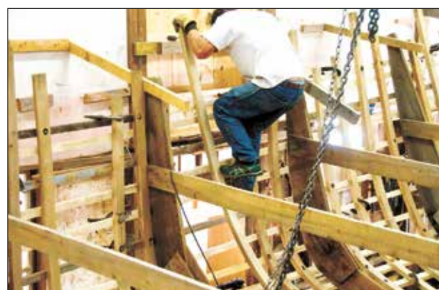
The lower end of the hot rib is driven into the pocket slot in the keel. Standing on the rib and pulling down on the end presses it against the lower ribbands first while it is being clamped to the ribbands.
