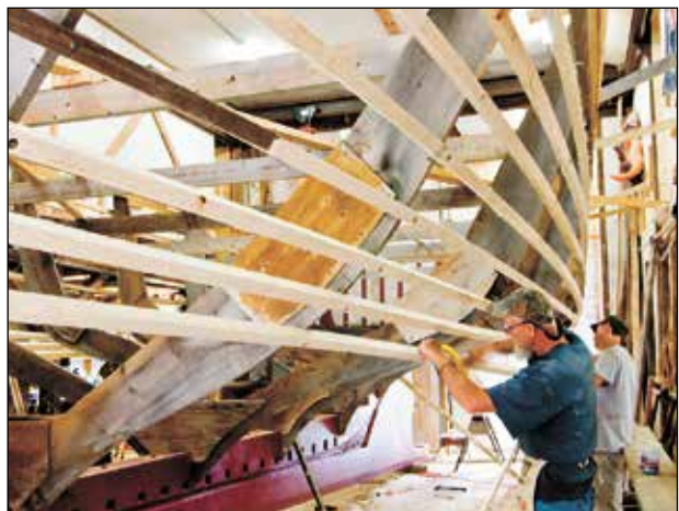
After all the molds are in place, ribbands are screwed to the molds to create a surface against which the ribs of the hull will be bent. The molds and the ribbands together are the form the hull will take it's shape from. After the ribs are bent in to place, the ribbands are gradually removed as the planking is done.
