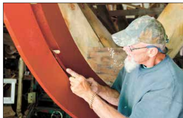
An important detail in a wooden boat are stop waters. These white cedar dowels are driven through holes wherever a keel seam, the joint between two parts of the keel, crosses the rabbet, the notch into which the hull's planks are set. The stop waters swell to block passage of water through the keel seam into the boat. The line of the keel seam may be visible here at a steep angle to the left of the white stop waters being saun flush with the rabbet.
