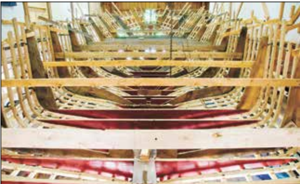
At this angle the only part of the keel visible now is the stem in the background. The molds, ribbands, ribs and red floors are all in position. Note the stabilizer braces nailed to the molds and the walls left and right.
