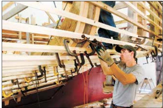
While one crew member forces down the hot rib from the inside (above), Jeff Hanley clamps the rib to a ribband.
