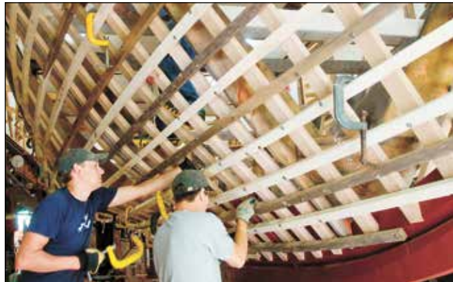
Andy Dickens, left and Jeff Hanley in the final stages of getting the molds, ribbands and ribs in place before planking begins.
