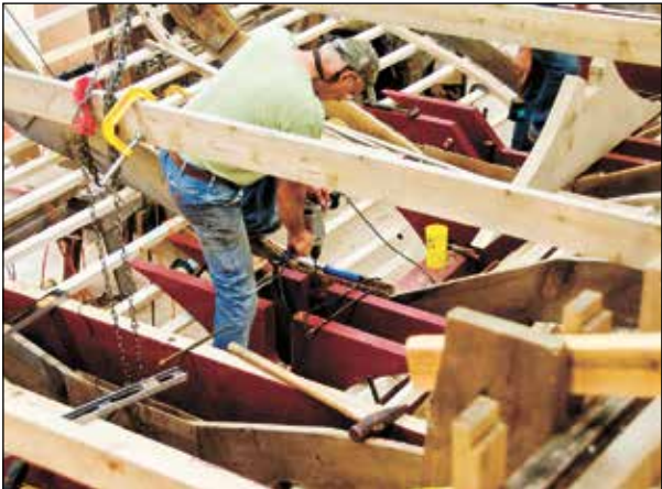
Several floors (dark red), each a unique shape based on the shape of the hull section, are attached to the keel. Here Sam Jones is drilling holes for driving metal drift pins that fasten the floor to the keel. Later planks will be fastened to the lower edges of the floors. The shaft passes through the floor being drilled. The two floors under Sam, the two in front of him with cutouts for the engine and the one behind him will carry the two parallel 14' x 4-1/2" x 7" white oak engine beds.
