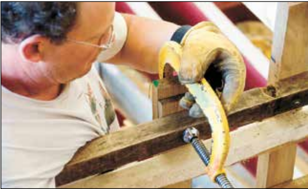
Ribs bent into a tight radius are split for half their upper length. The difference between the inner and outer radius is visible in the the ends of the two halves being clamped to a ribband. This technique avoids stress cracks in the rib later.
