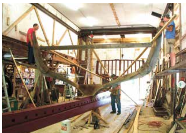
The first mold in place on the keel. Measurements taken off the keel (aft) position it properly. The wood braces from the upper left and right sides of the mold to the keel are nailed to hold the mold in place.
