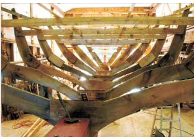
The first seven of the twelve molds tacked in place. On this 46 footer they are about 40" apart. The keel is set up to sit as it would in the water. The waterline will then be level. The molds are squared to the keel and then made plumb.
